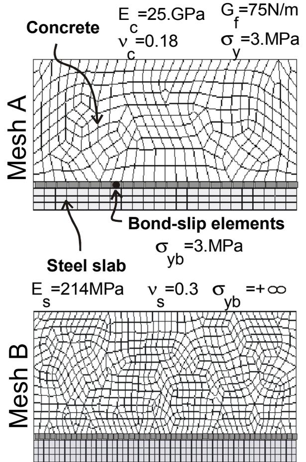
Figure 16. Steel slab in a concrete block. Finite element meshes.
