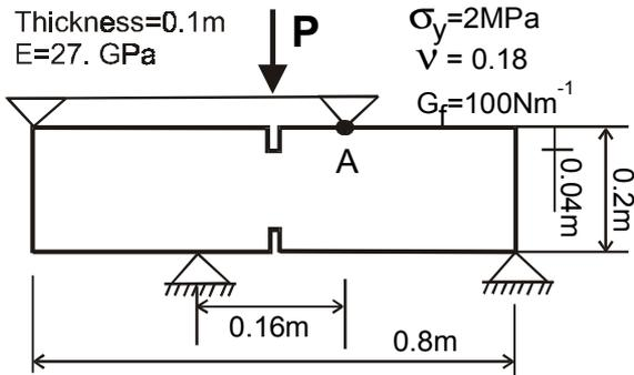
Figure 10. Four-point bending test for a double-notched beam, E: Young' modulus, v: Poisson's ratio,  $\sigma_y$ : tensile strength.  $G_f$ : fracture energy
