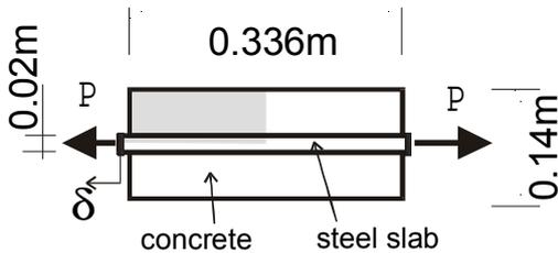
Figure 15. Debonding of a steel slab from a concrete block in plane strain. The discrete model corresponds to a quarter of the structure.
