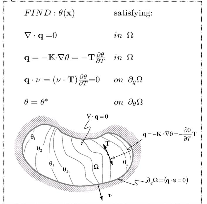
Figure 6. 2D algorithm to compute the envelopes of the propagation field as the isothermal lines for a heat conduction problem.
