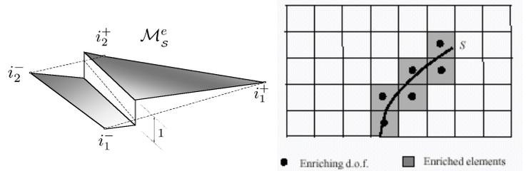
Figure 2. Elemental based enrichment. Left: discontinuous enriching displacement mode. Right: enriched domain crossed by the discontinuity path
