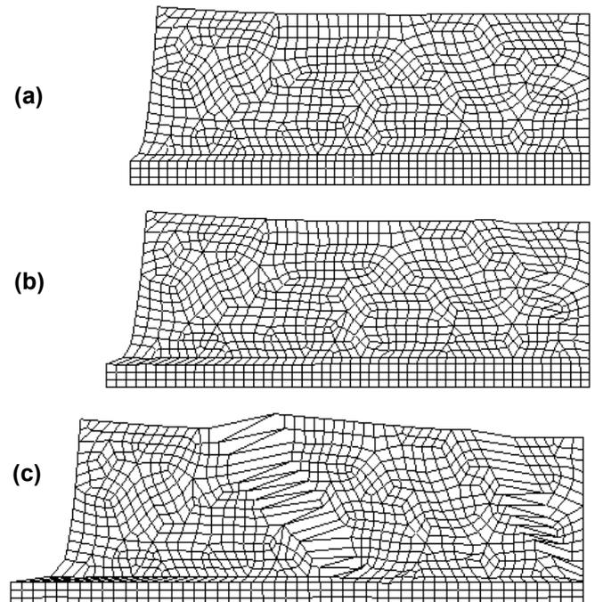
Figure 19. Steel slab in a concrete block. From (a) to (c): Deformed (amplified) meshes at identical times than in Figure 18.
