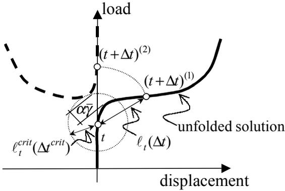
Figure 9. Algorithmic bifurcation for the unfolded problem. For  $\ell_t(\Delta t) > \ell_t^{crit}(\Delta t^{crit})$  the algorithmic solution may not be unique.
