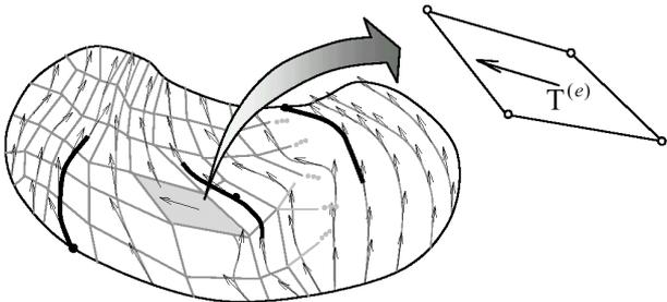
Figure 5. Discontinuity tracking in a 2D problem using a global algorithm. The algorithm traces the envelopes of the propagation vector field  $\mathbf{T}(\mathbf{x}) \perp \mathbf{n}(\mathbf{x})$  and then selects some of them as propagating cracks.
