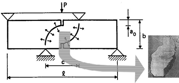
Figure 11. (from Bocca P., Carpintieri A., Valente S., 1991) Four-point bending test for a double-notched beam, Left: observed cracks. Right: detail of the concrete specimen between cracks after the test.
