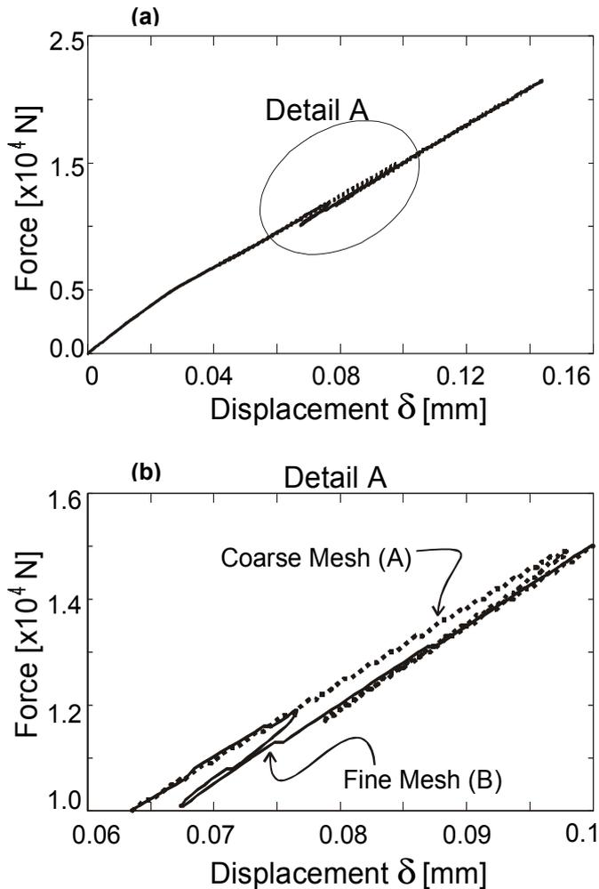
Figure 17. Steel slab in a concrete block; (a) Load vs. displacement curve at the end-face of the slab; (b) detail of the curve showing the snap-back caused by the complete softening of the primary crack.
