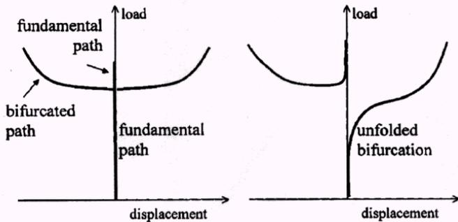
Figure 7. (from Gastebled et al. 2000): Bifurcation unfolding. Left: unperturbed solution. Right: perturbed solution
