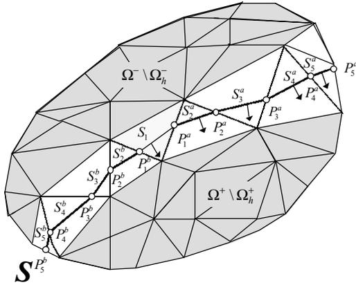
Figure 4. Discontinuity tracking in a 2D problem using a propagation algorithm: The original segment  $S_1$  in the root element propagates in both senses by means of straight elemental segments  $S_i^a$  and  $S_i^b$ .
