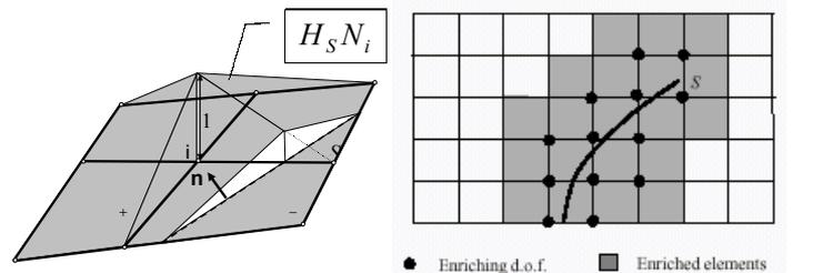
Figure 3. Nodal based discontinuous enrichment. Left: discontinuous enriching displacement mode. Right: enriched domain crossed by the discontinuity path
